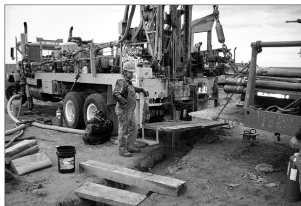
The drill rig is the key tool for exploration of uranium deposits. It holds equipment for drilling holes through rock and collecting samples and logging geologic data. [Source: Strathmore Minerals web site]
