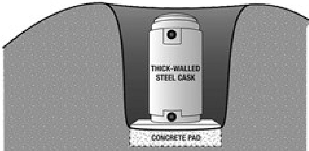
Nuclear rods cooled by simple air convection.
