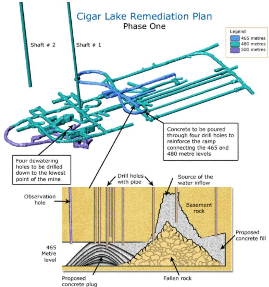
10 drill holes are needed for concrete pouring and grouting to remediate the area of the rock fall and water inflow
