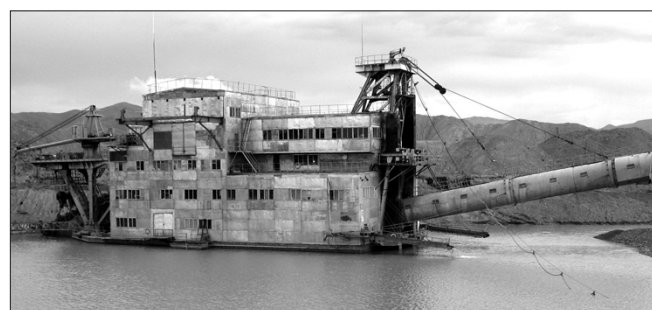
Large bucket dredges are used to extract gold placer ore at gold mines in the floodplain of the Tuul River in Mongolia.
