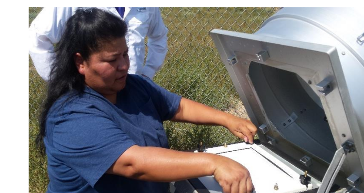
Community member Tiva Shirley operates a particulate matter (PM) collector in 2015 as part of a study of metals in dusts released from abandoned mine sites.
