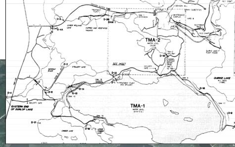
Denison tailings – 63 million tons - are placed in preexisting lakes with man-made perimeter dams
