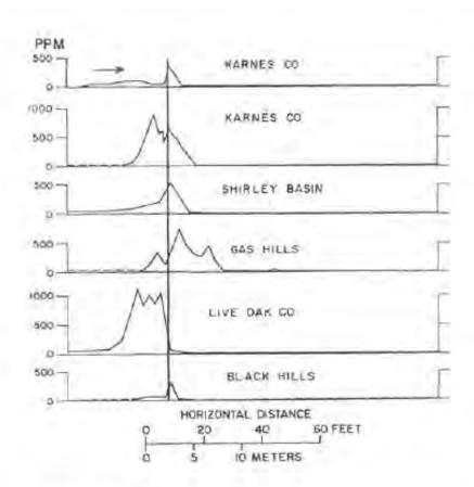
Figure 6. Concentration and distribution of selenium in various uranium roll from deposits (after Harshman, 1974).
