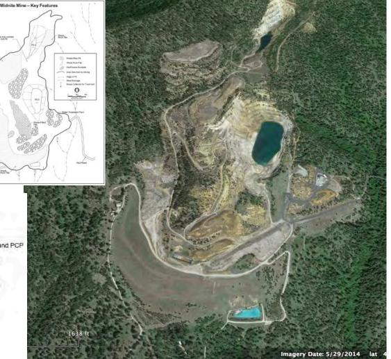
Midnite Mine remediation cost of \$193 million shared by Newmont Mine (72%) and US Government (28%).Completion of Remedial Plan due 2025, perpetual treatment of 5 – 10 million gallons of mine pit and seepage water at on-site plant requires treatment plant with 26 million gallons/year to manage peak flows. and disposal site for 40-80 tons of mine water treatment sludge required.
