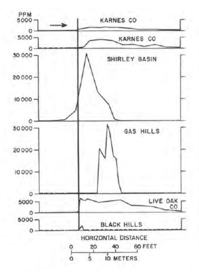
Figure 8. Concentration and distribution of arsenic in various uranium roll front deposits (after Harshman, 1974).
