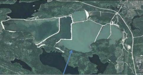
Quirke – 46 million tons – tailings surrounded by manmade dams and internal dykes with built on tailings, with inflowing water cover water at 5 elevations.
